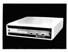
System compatability, the ability to exchange data with existing Packet Terminal Node Controllers, has been achieved with the Kantronics Packet Communicator by using the popular TAPR software.
